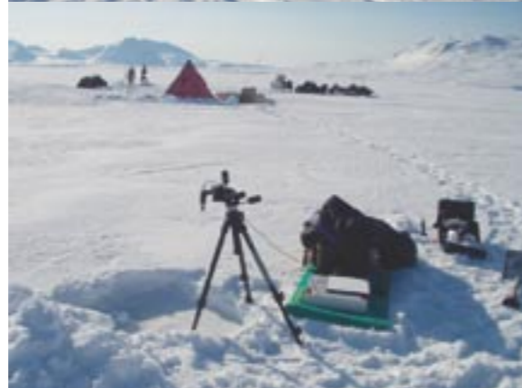
The setup for surface reflectance measurements in the field (here in April 2003 on Kongsfjorden). The downlooking optical sensor on the tripod is connected with an optical fibre to the spectroradiometer.
