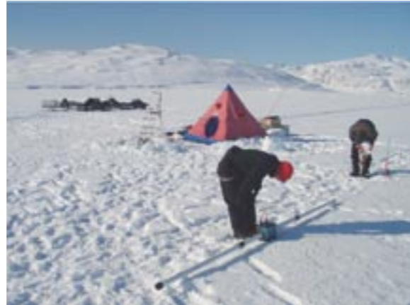
The AIO research site on the fast ice of inner Kongsfjorden, Svalbard. Foreground: electromagnetic ice thickness profiling. Background: tent for under-ice turbulence monitoring equipment and snow machines for travel between Ny-Ålesund and the research site.
