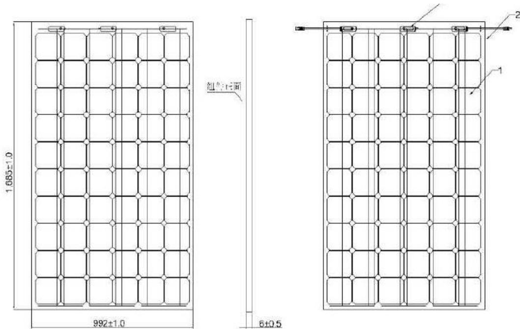
Figure 2-36 schematic diagram of solar cell component size
