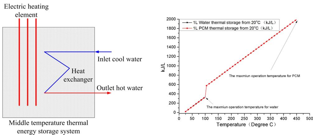
Figure 2-45 Schematic diagram of middle-temperature thermal energy storage system with PCM
