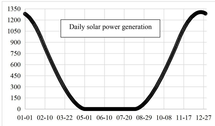
Figure 2-37 RSNRS 100kW Photovoltaic energy system annual power generation
