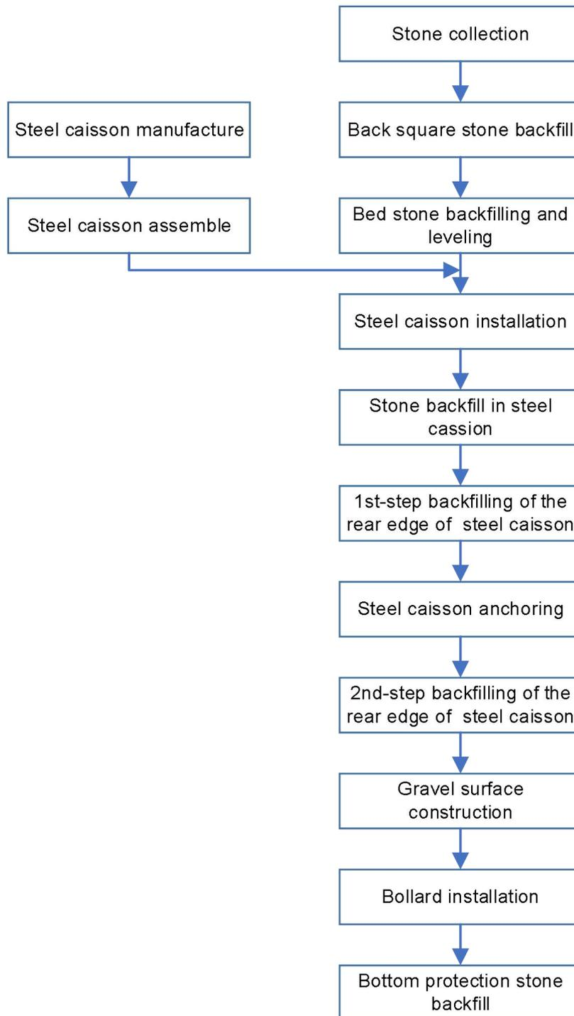
**Figure 2- 56 Consutruction process of the wharf area**
