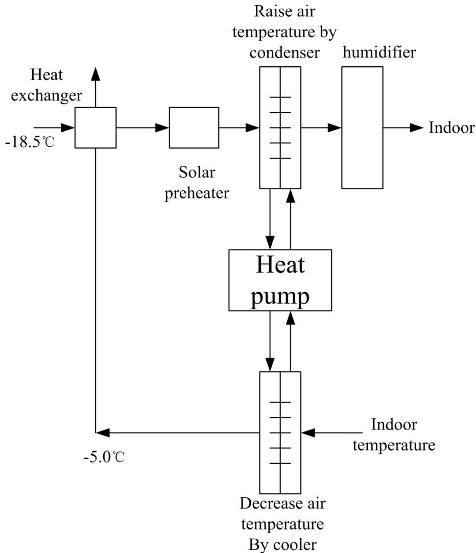
Figure 2- 48 Schematic diagram of fresh air preheating system
