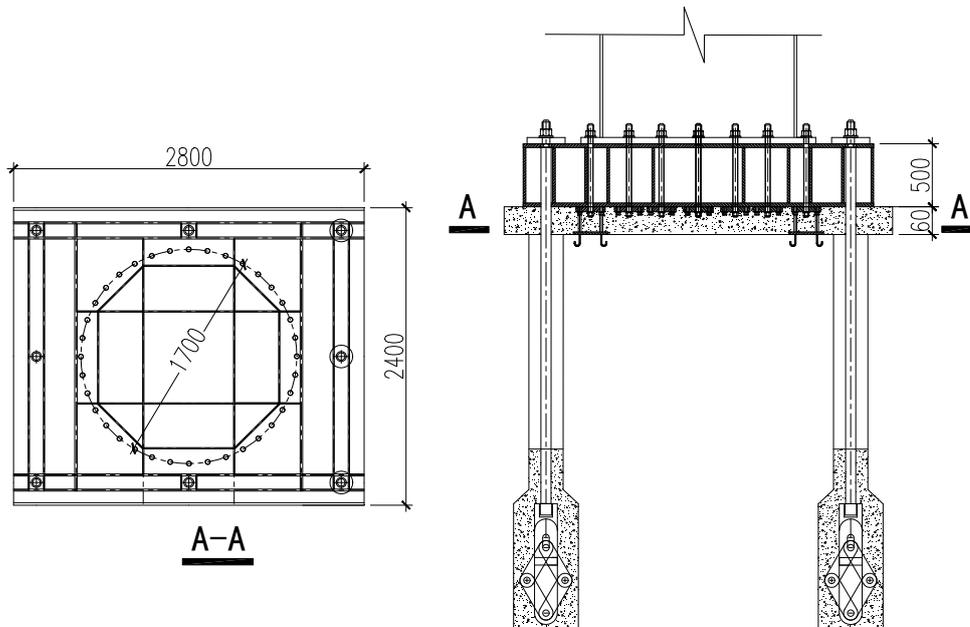
Figure 2-50 Rock anchor bolt foundation sketch (Unit: mm)
